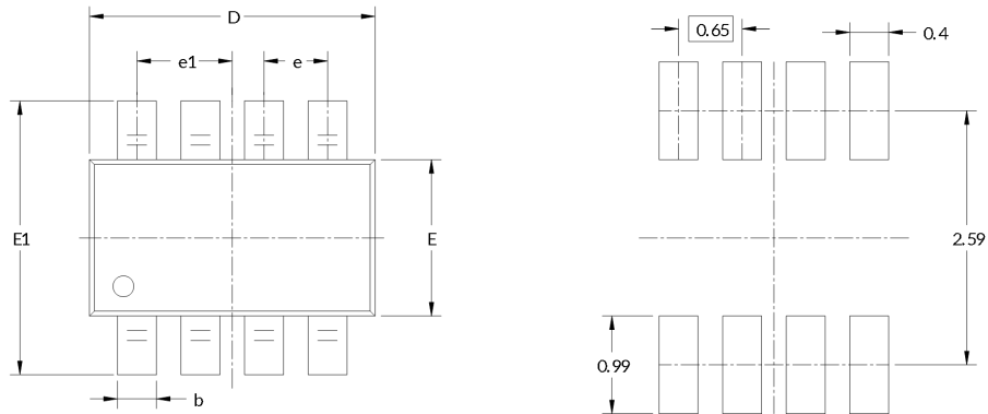
RECOMMENDED LAND PATTERN (Unit: mm)
